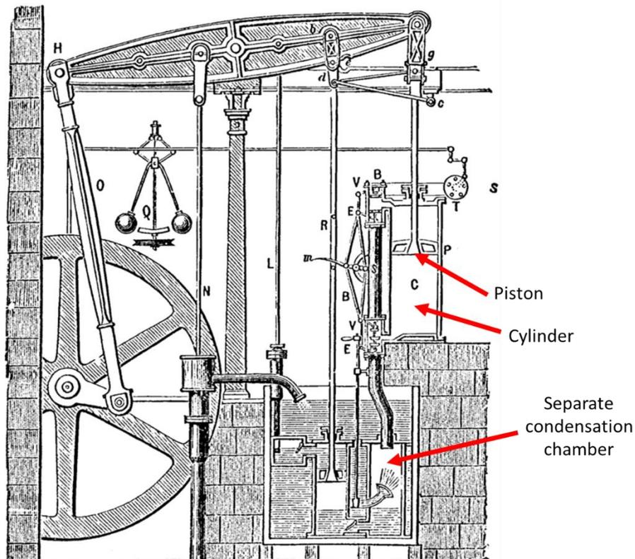
Watt's genius was to realise that the Newcomen engine wasted almost three quarters of the energy in the steam through heating the piston and cylinder. With a separate condensation chamber, efficiency was more than doubled. As the cost of the machine was similar, the energy produced was much cheaper.
