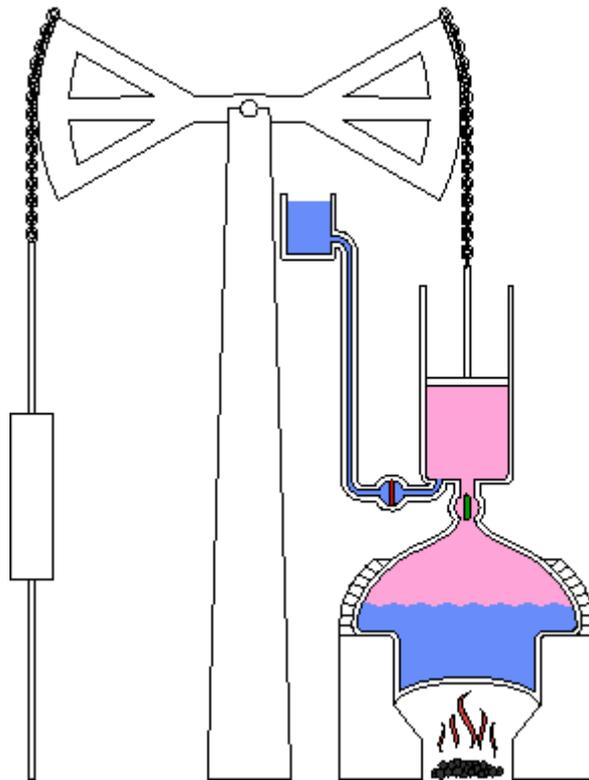
With this [heat engine](#), humans were finally able to convert thermal energy into mechanical energy, marking the start of the [industrial revolution](#).
